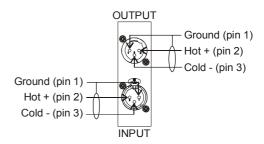
If using the unit with unbalanced signals (not recommended), then connect the input between Hot+ (pin 2) and ground (pin 3), and connect the Cold- (pin 3) input to ground. Take the output from Hot+ and ground, and leave Cold- (pin 3) unconnected. Note that when using unbalanced input connections the gain is reduced to -6dB.
