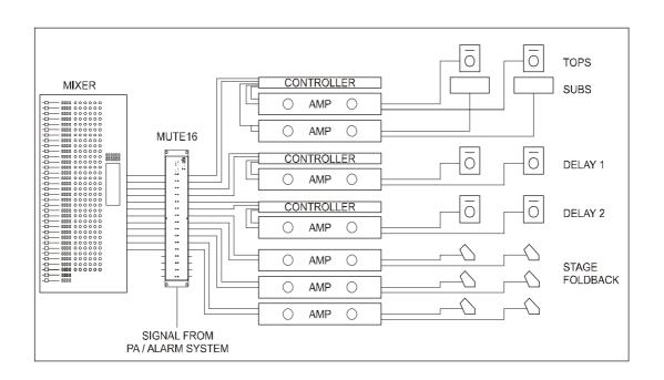
The Mute16 uses voltage controlled amplifiers to shape the amplitude of the signal in order to avoid switching clicks, and to provide a gradual return ramp of the signal when the mute is lifted. The control signal is a simple switch contact that is optically isolated within the Mute16.
